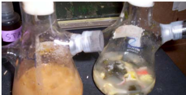
Fig. 4 Batch SSF experiments of food waste
